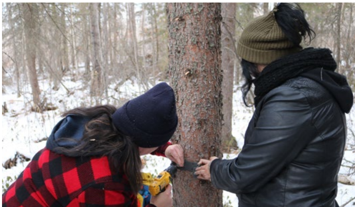
Cameras are mounted in metal brackets drilled to trees to ensure they remain aimed at the targeted site location.
